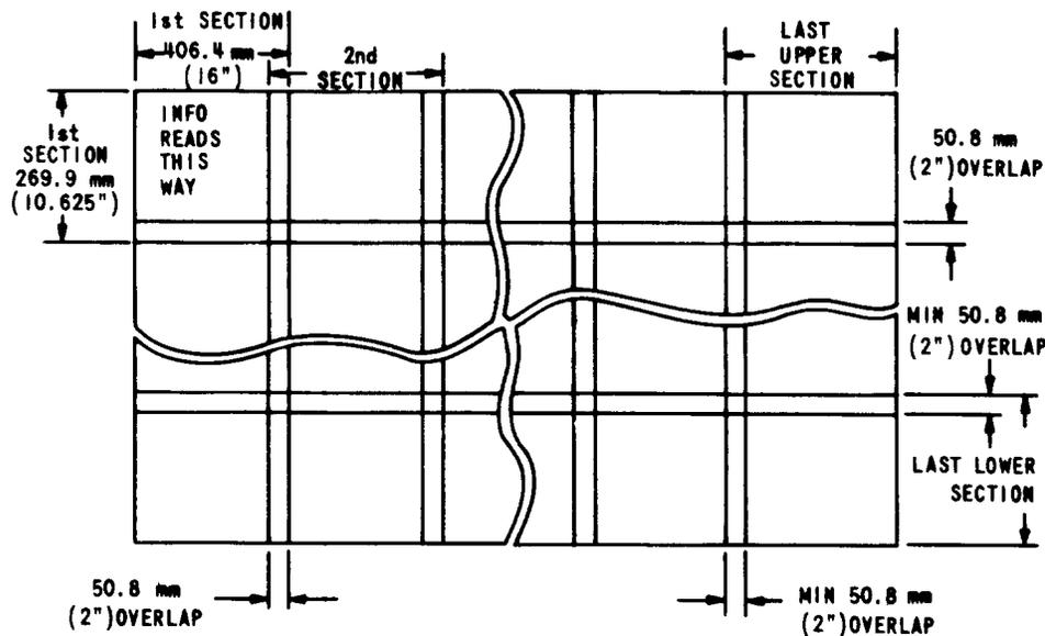
Fig. 8—Sectionalizing of Information Areas for Multiple Double Frames [Over 269.9 mm (10.625 Inches) High]
