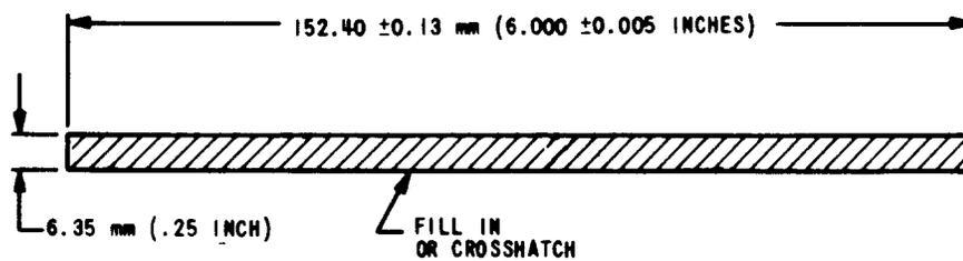
**Fig. 11—Reduction Test Strip Dimensions**
