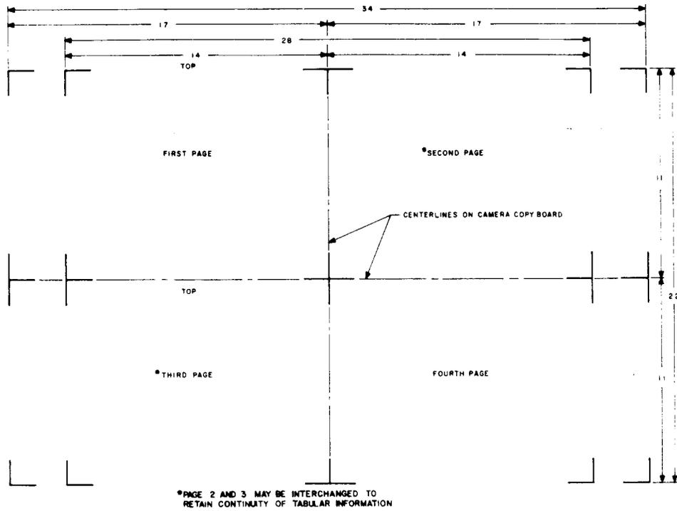
**Fig 10—Layout for 14 by 11-Inch and 17- by 11-Inch Pages**
