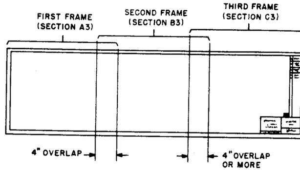
Fig 7—Multiple-Frame Drawing
