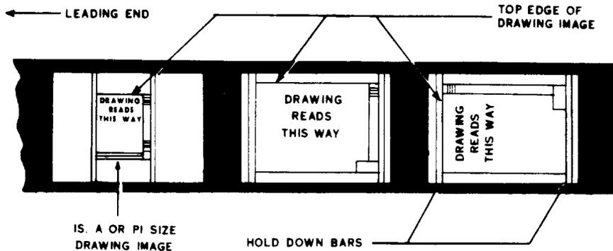
Fig 14—Single-Frame Drawing Image Orientation
