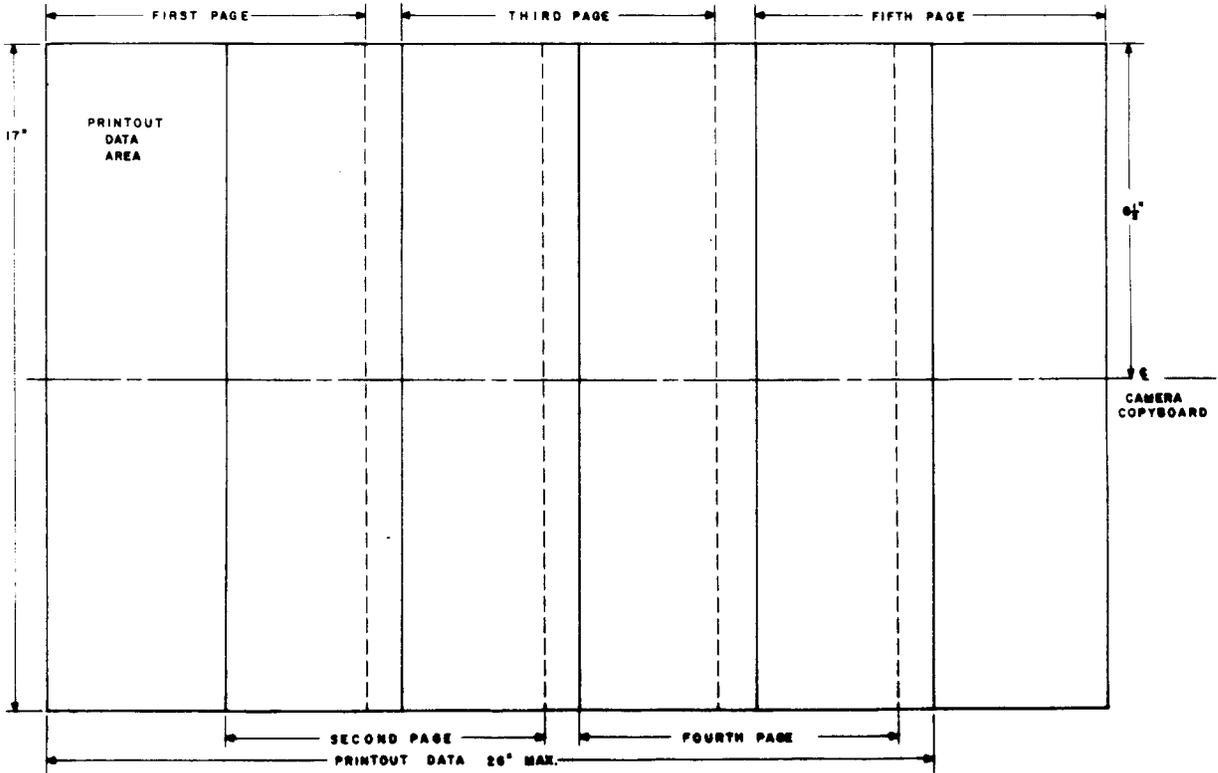
**Fig 13—Layout for up to Five 9-3/8 by 17-Inch Computer-Generated Pages**
