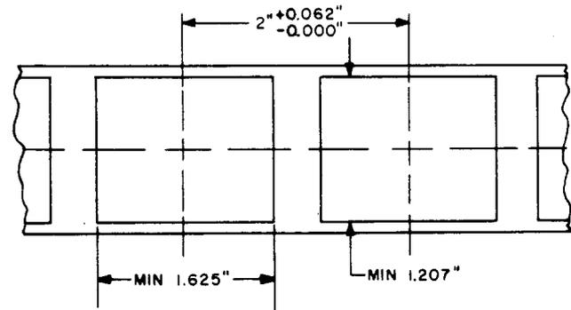
**Fig 5—Microfilm Frames**
