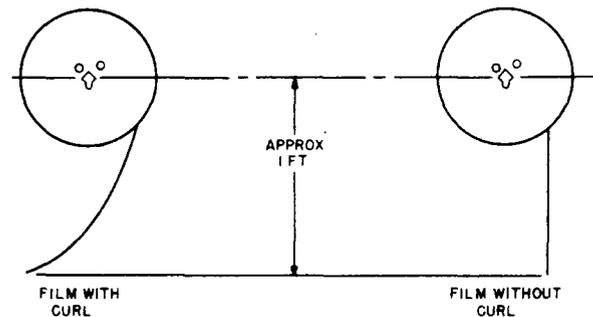
**Fig 16—Checking Reel Film for Curl**
