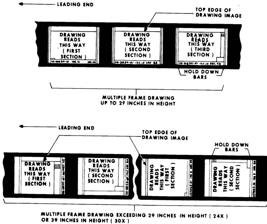
Fig 8—Multiple-Frame Drawing Section Image Orientation
