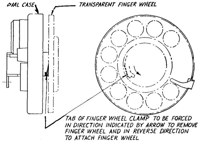
Fig. 10—Tab of Finger-Wheel Clamp
