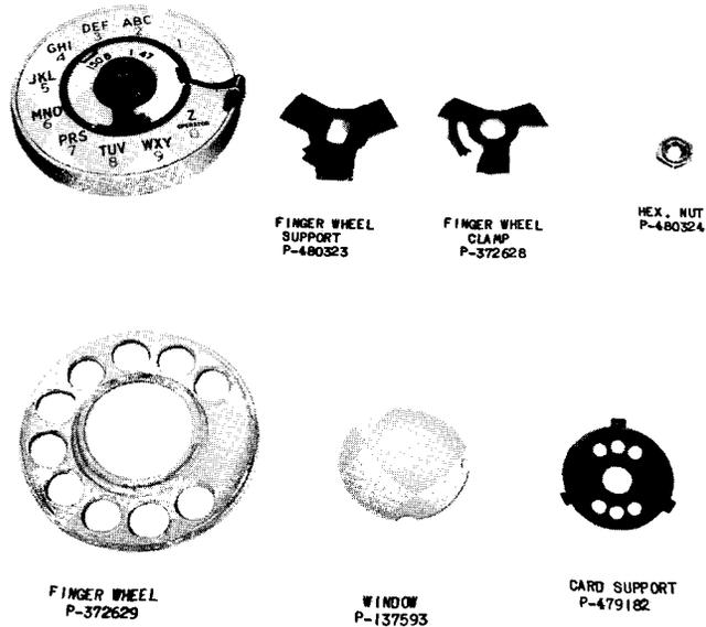
Fig. 11—P-335580 Finger Wheel Assembly
