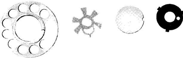
Fig. 13—P-13A106 Finger-Wheel Assembly for 6- and 7-Type Dials
