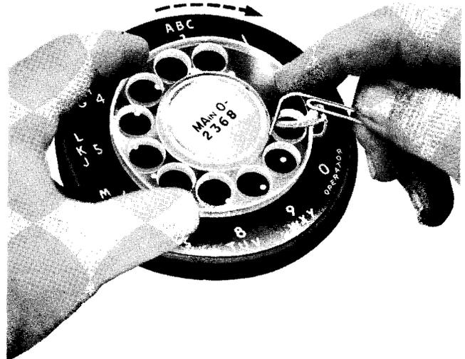
Fig. 14 -Removing Plastic Finger Wheel
