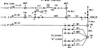
Fig. 12-872A1M Telephone Set-2/4 Wire Connections
