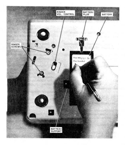
Fig. 6-872A1M Telephone Set, Bottom View
