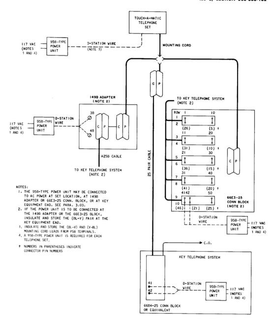
Fig. 7-872A1M Telephone Set, Alternate Power Connection Method
