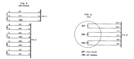
Fig. 8-872A1M Telephone Set, Connections (Sheet 2 of 4)
