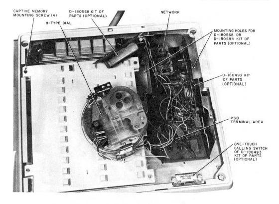
Fig. 4—872A1M Telephone Set—Dial Removed To Show Terminal Area
