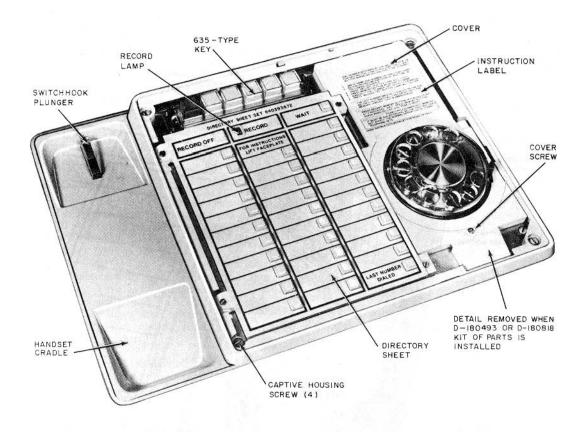
Fig. 2—872A1M Telephone Set—Faceplate and Handset Removed
