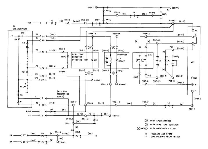
Fig. 14—872A1M Telephone Set, Partial Functional Schematic
