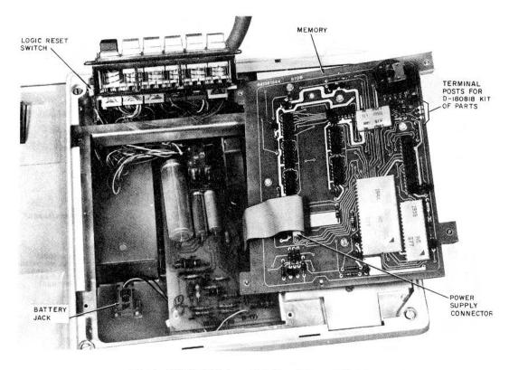
Fig. 5-872A1M Telephone Set, Overall Internal View
