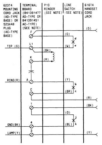
NOTE: THIS PARTIAL DRAWING SHOWS HOW A TELEPHONE SET BASE MANUFACTURED AFTER 6-1-82 AND MARKED FOR "1-PTY" SERVICE CONNECTIONS IS WIRED IF IT IS EQUIPPED WITH ALL THE ABOVE LISTED COMPONENTS. A SET CAN BE MARKED "1-PTY" WITHOUT HAVING ALL THE LISTED COMPONENTS. IF THIS ARRANGEMENT IS ENCOUNTERED, REFER TO FULL SCHEMATIC DRAWING OF THE TELEPHONE SET AND PARAGRAPH 2.14 (a) THROUGH (c) TO COMPARE DIFFERENCES IN THE WIRING.
