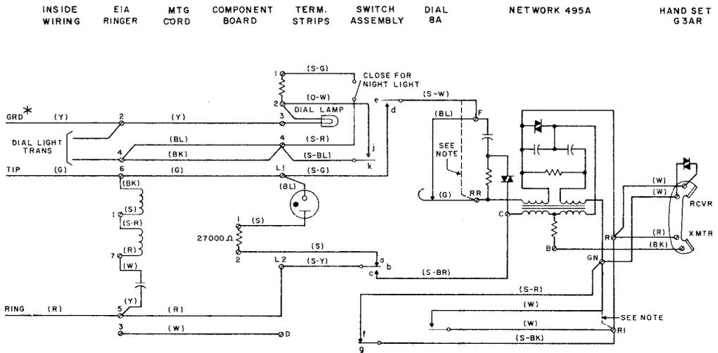
Note: For manual service, remove lead from Terminal F and connect to RR and remove white dial lead from Terminal GN and connect to R1.
