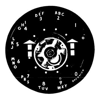
Fig. 7 — Lock Ring Removal
