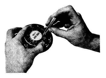
Fig. 4 — Removing Plastic Fingerwheel
