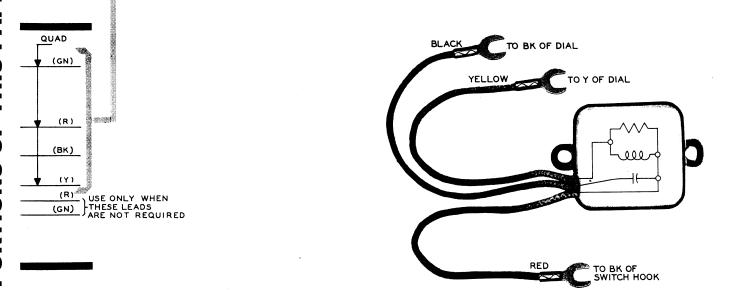
Fig. 7—61M FILTER CONNECTIONS
