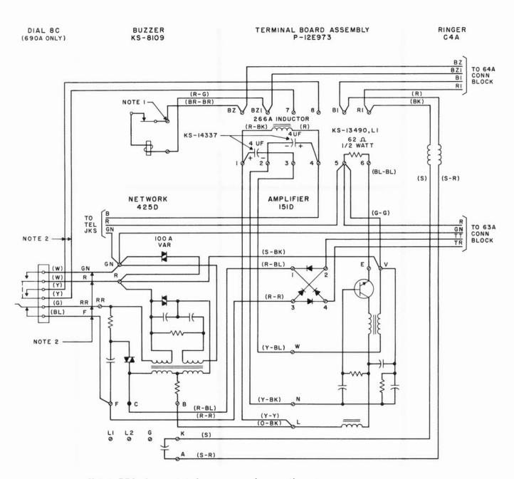
Note 1: BZ lead connects to buzzer case under mounting screw.
