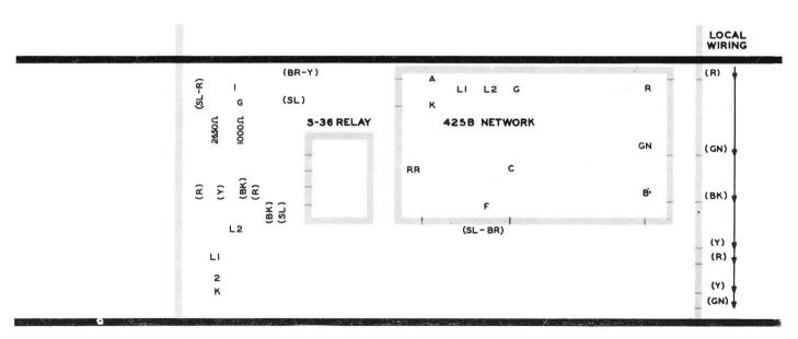
Fig. 1 — Circuit Diagram for Connection with Coin Collectors
