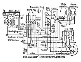
Note 1: If filter is not provided, connect yellow lead from Y of switchhook to Y of dial instead of to filter bracket terminal.
