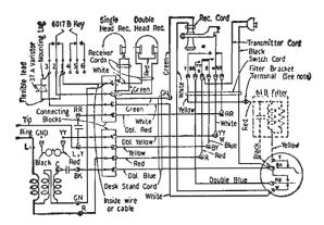
Note 1: If filter is not provided, connect yellow lead from Y of switchhook to Y of dial instead of to filter bracket terminal.
