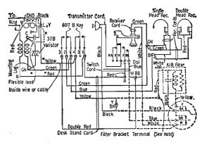
Note: If filter is not provided, connect yellow lead from terminal 4 of key to Y of dial instead of to filter bracket terminal.
