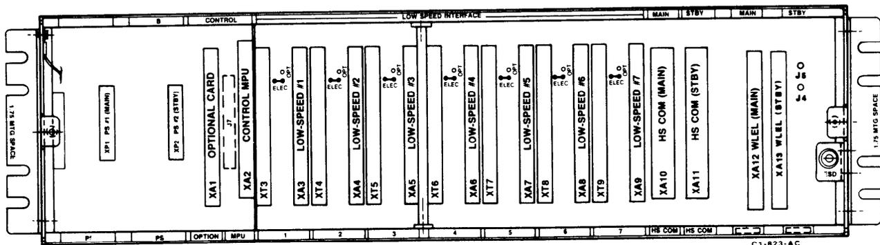
Figure 2E-1. Front of 828A Digital Multiplexer (Cover Removed)
