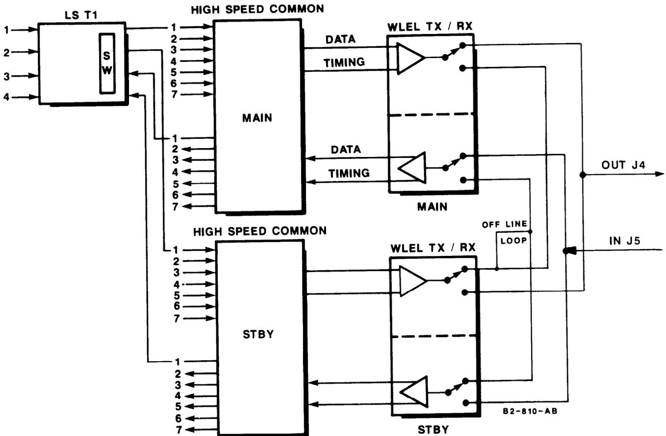
Figure 2-2. 828A Digital Multiplexer Block Diagram
