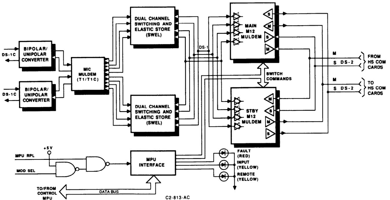
Figure 2A-4. LS INTER T1C Card Block Diagram
