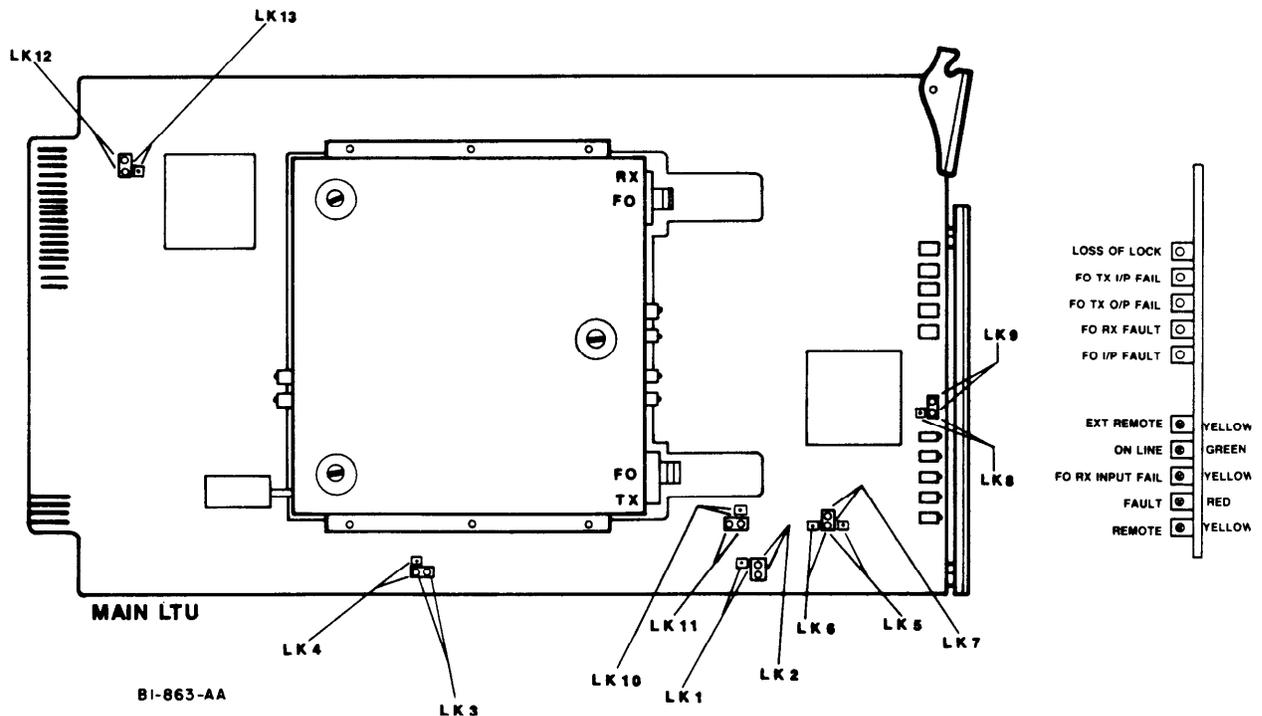
Figure 2C-1. LTU Low-Speed Interface Card (MAIN LTU Illustrated)
