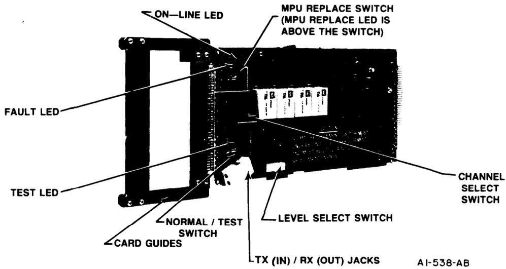
Figure 2-5. Maintenance Interface Card
