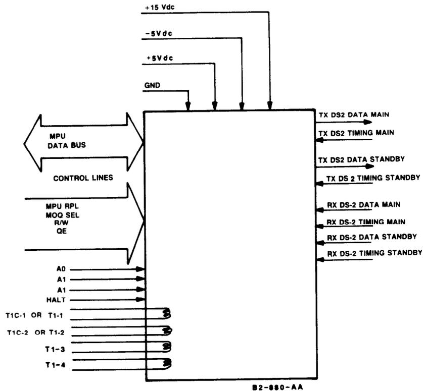
Figure 2A-2. LS INTER T1/T1C Card Interfaces
