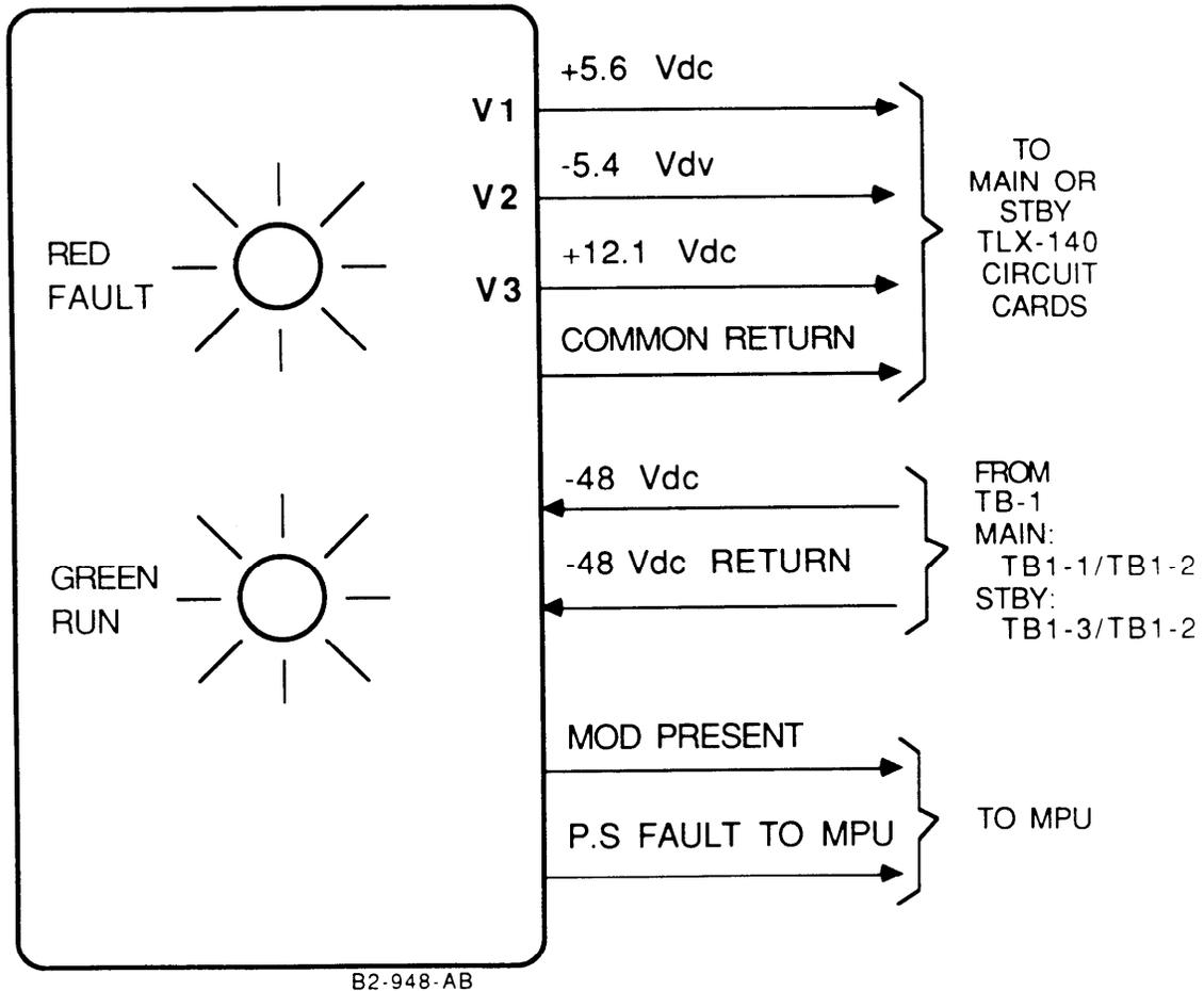
Figure 2H-2. PS Module Interfaces
