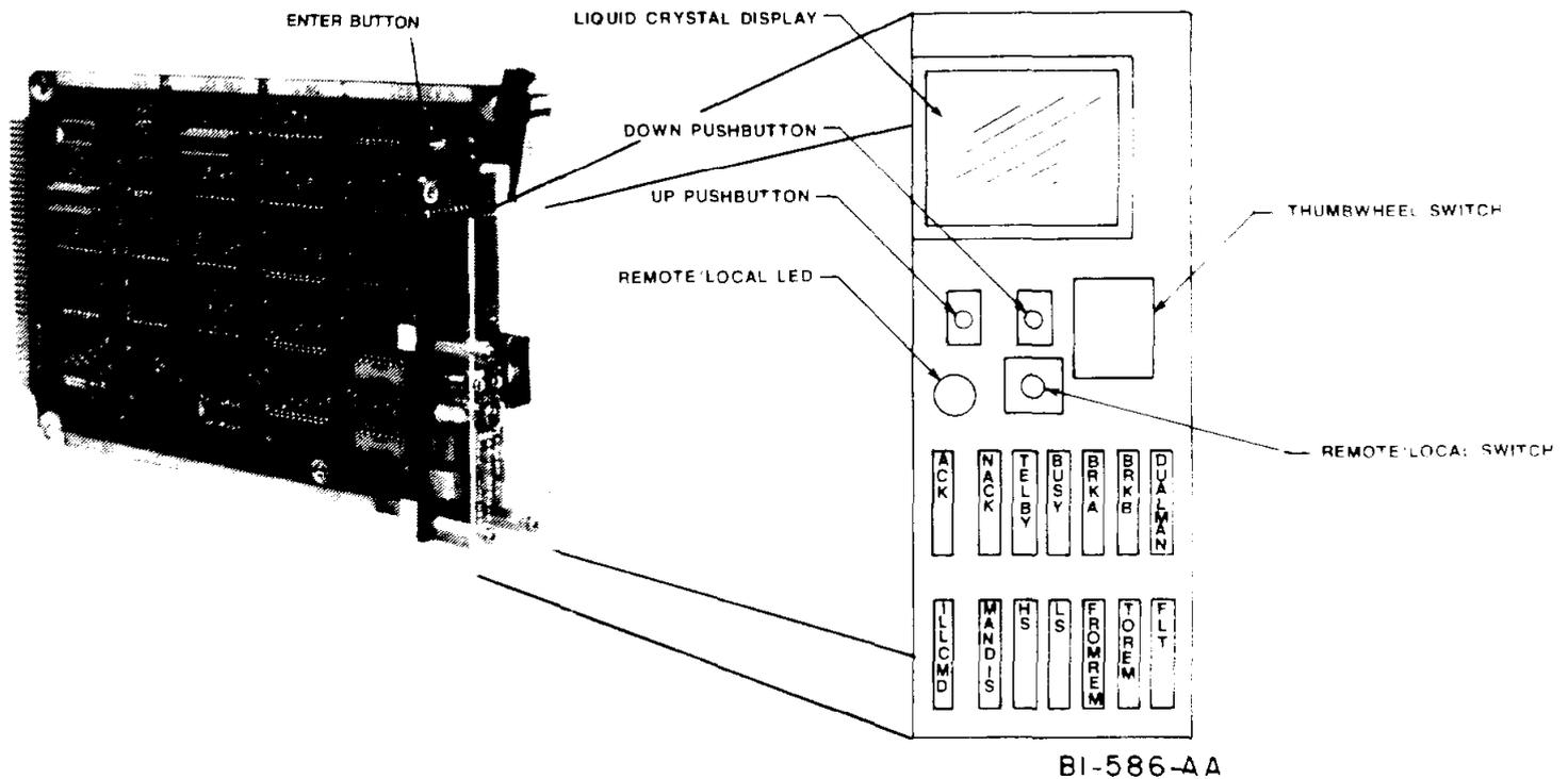
Figure 2-7. Manual Control Interface Card
