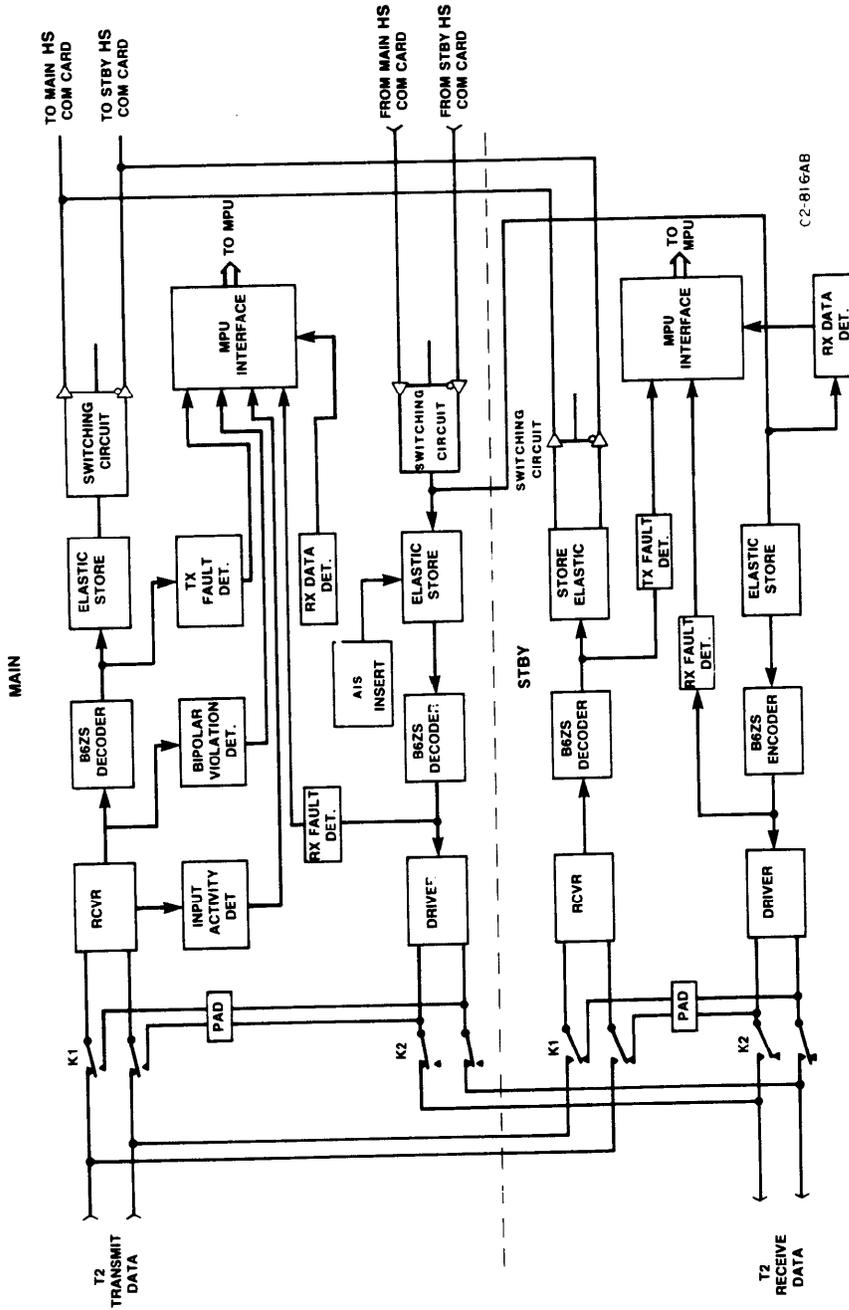
Figure 2B-1. LS INTER T2 Card (MAIN and STBY) Block Diagram
