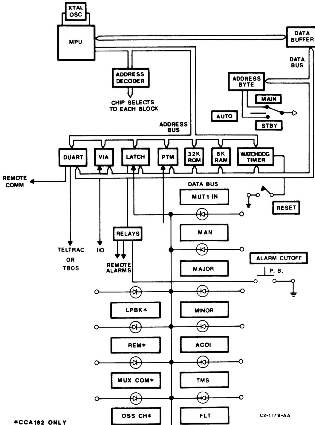
Figure 2F-3. Control MPU Card Block Diagram
