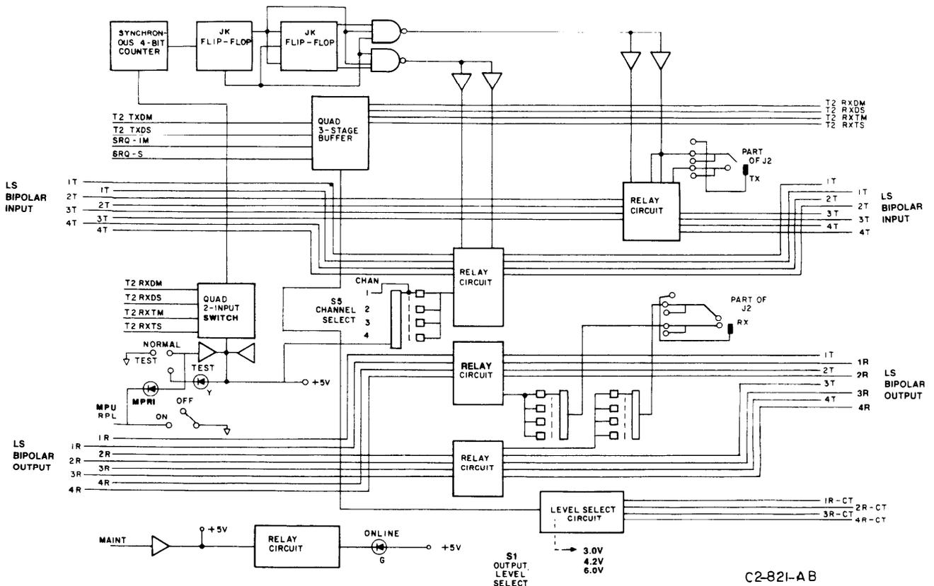
Figure 2-6. Maintenance Interface Card Block Diagram
