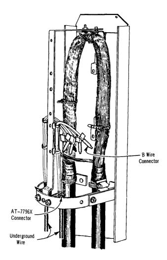
Fig. 5 – D Underground Wire in 38-Y-D and 38-Y-DB Cable Closure
