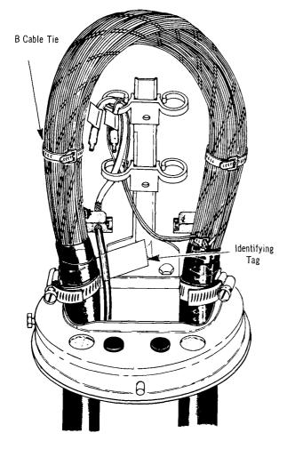
Fig. 3 – Underground Wire in B Cable Closure
