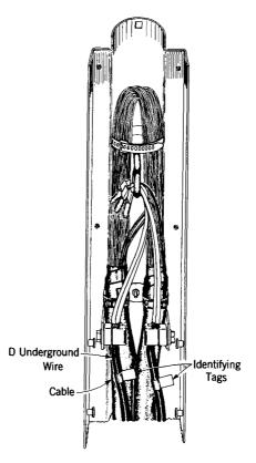
Fig. 7 – D Underground Wire in D Cable Closure
