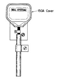
Fig. 12 - Protector With Cover in Place
