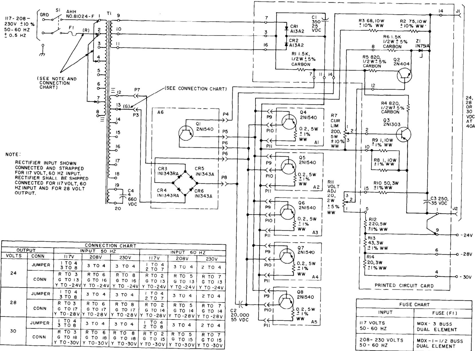
Fig. 3—KS-19231 L2 Rectifier Simplified Schematic
