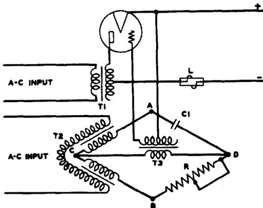
Fig. 3 - Phase Shift Control - Half Wave - Manual
