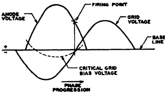
Fig. 2 - Voltage Relations - Phase Shift Control of Firing Point
