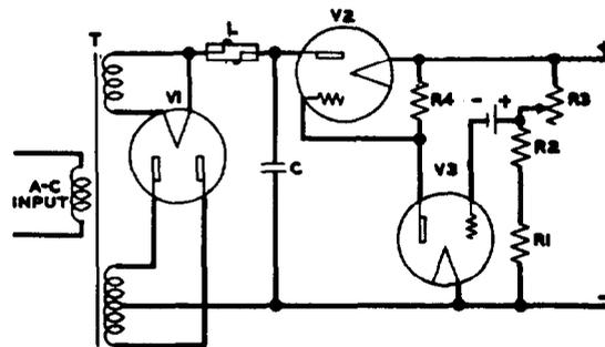
Fig. 8 - Series Tube Control - Full Wave with Grid Battery
