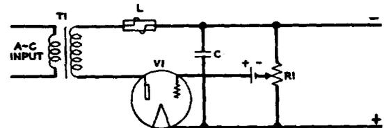
Fig. 6 - Magnitude Control - Half Wave
