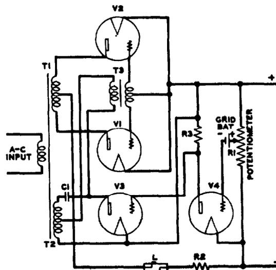
Fig. 4 - Phase Shift Control Full Wave - Automatic
