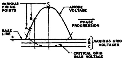
Fig. 5 - Voltage Relations - Magnitude Control of Firing Point
