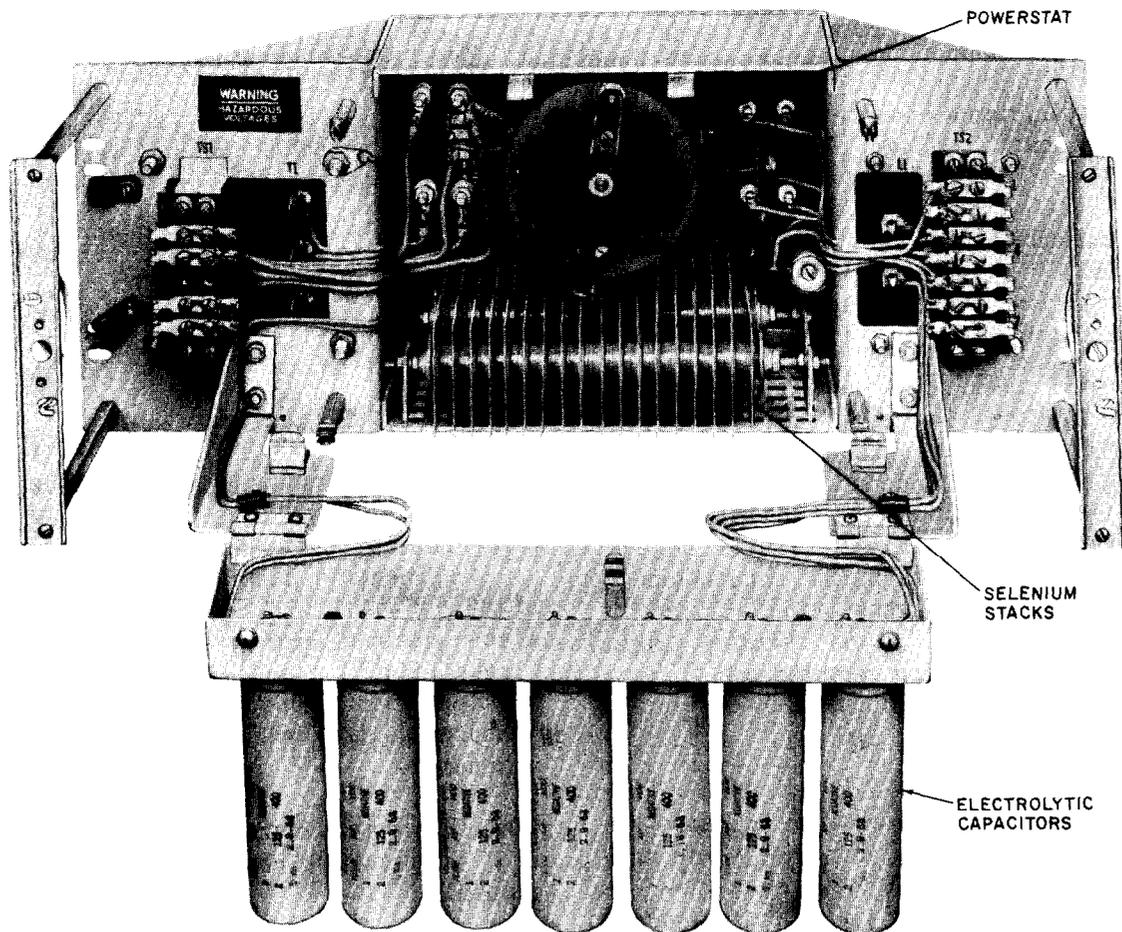
Fig. 3—J86254B, List 1 Rectifier—Rear View—Cover Off
