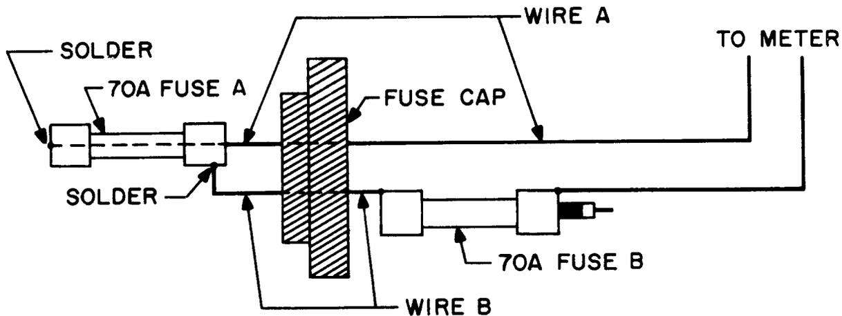
Fig. 1 - Construction of Dummy Fuse for Charge Current Measurements
