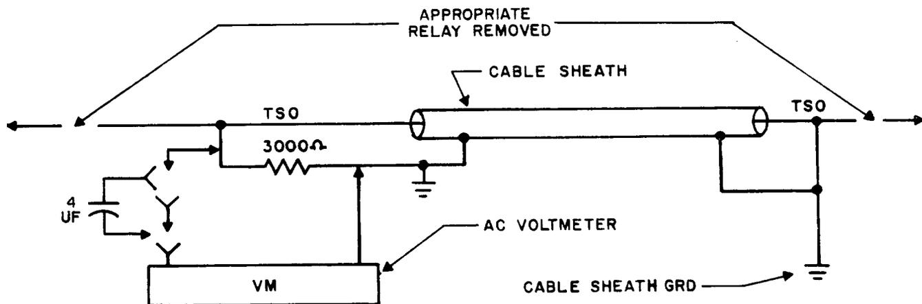
Fig. 4 - Measurement of AC Interference on Signal Leads
