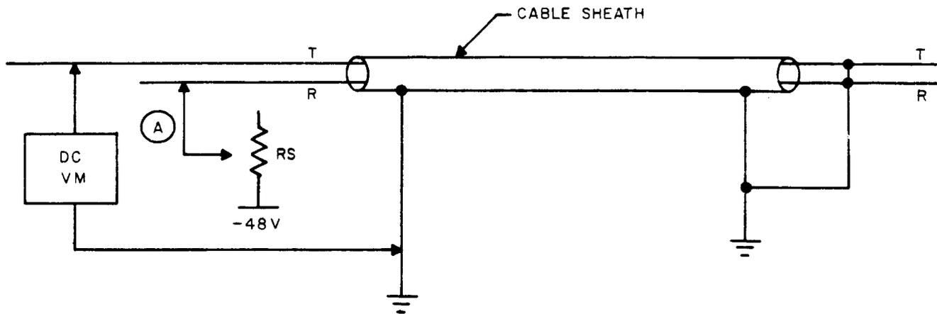
Fig. 2 - Measurement of Ground Return Resistance
