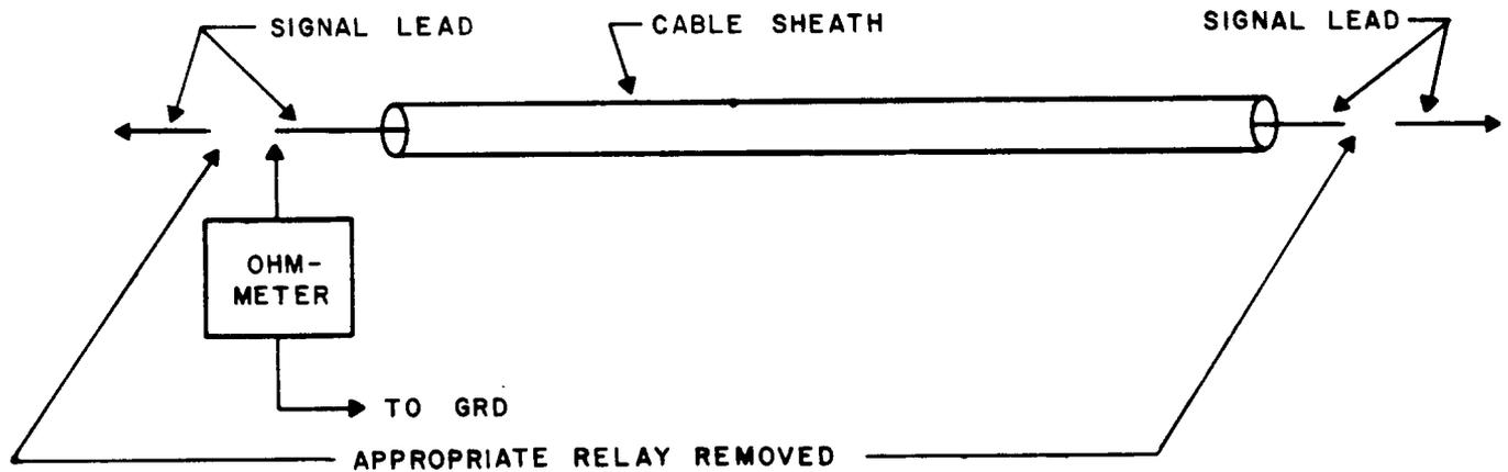
Fig. 3 - Measurement of Signal Lead Insulation Resistance
