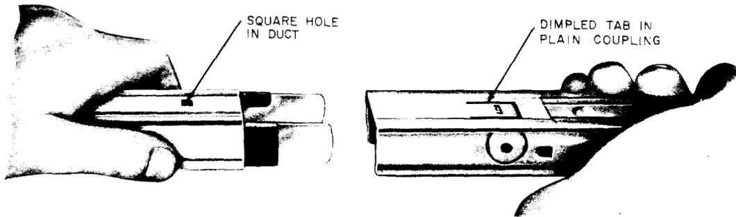
Fig. 11—Replacing a Duct Section
