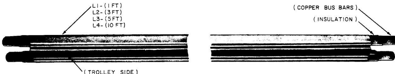
Fig. 1—KS-20085 Bus Duct, Trolley Type
