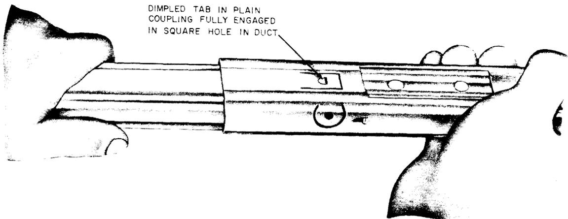
Fig. 12—Duct Coupling Fully Engaged
