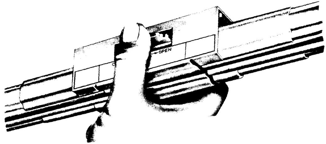
Fig. 15—Rotating Knurled Wheel of KS-20085 L6 Coupling
