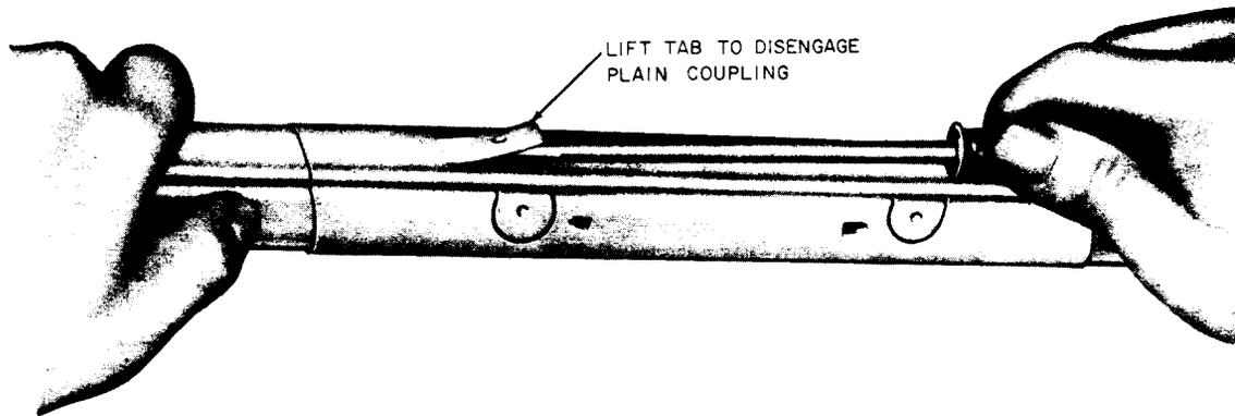
Fig. 10—Method of Disconnecting Duct Couplings
