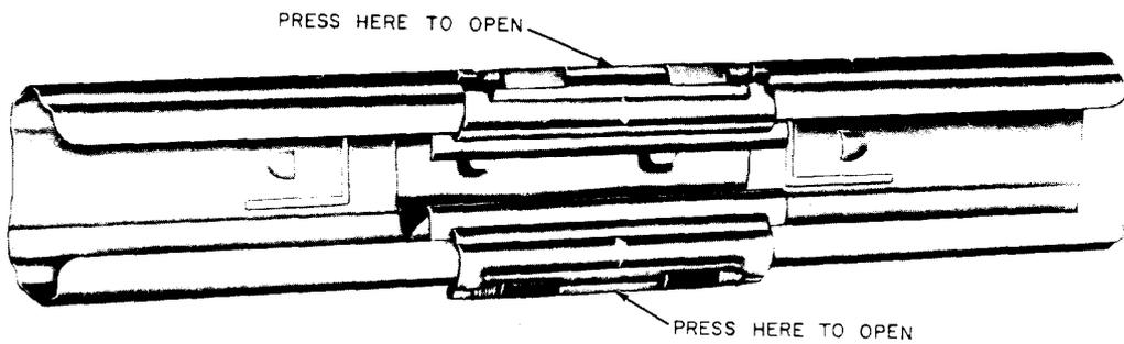
Fig. 13—Older Type Trolley Entrance Coupling (Closed)
