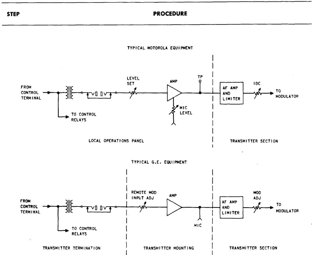
**Fig. 2—Typical Transmitter Input Arrangements**
