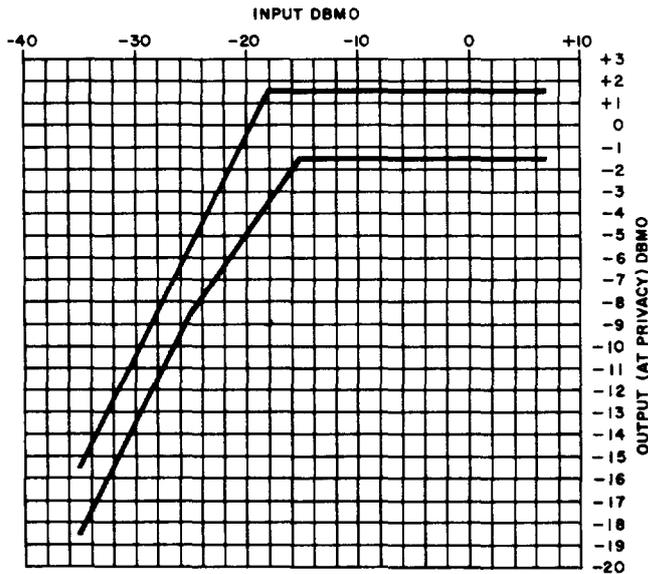
Fig. 5—Receive: Fading Regulator Characteristic Input/Output
