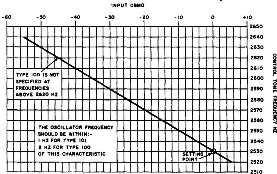
Fig. 4—Transmit: Input/Control Tone Frequency Characteristic
