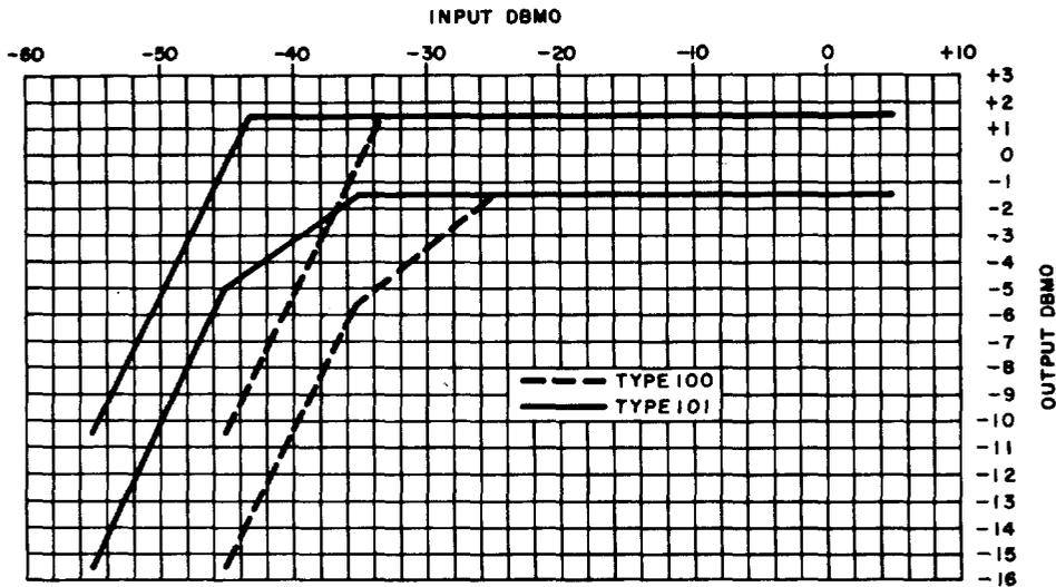
Fig. 3—Transmit: Compression Characteristic, Input/Output
