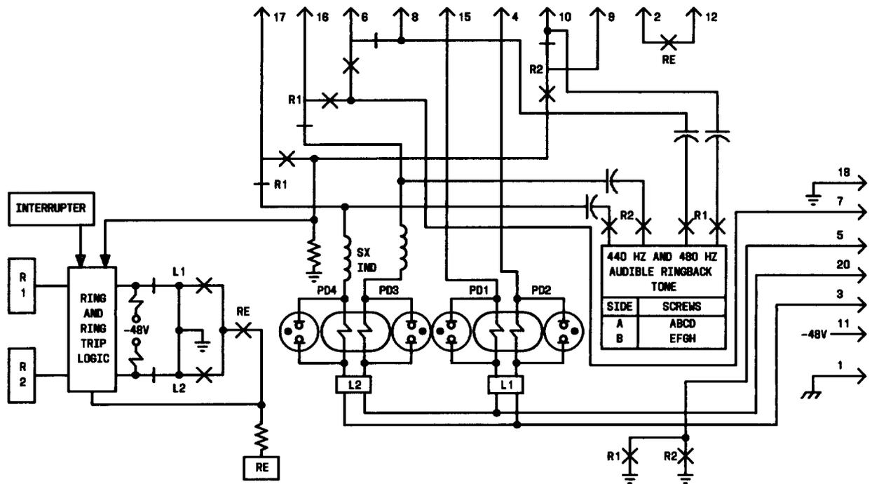
Fig. 1—J99343EC-1, L2 Block Diagram
