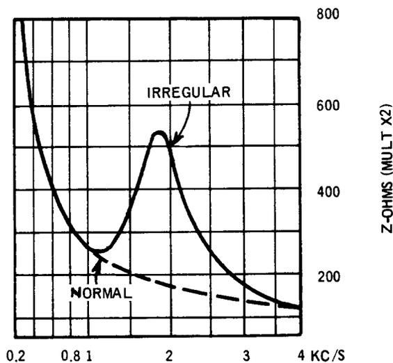
**Fig. 4 – Effect of Load Connected in Error on Open Circuit Nonloaded Pair Impedance**
