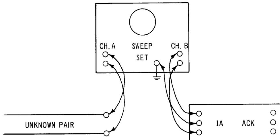
Fig. 2 - Arrangement for Impedance Comparison Technique
