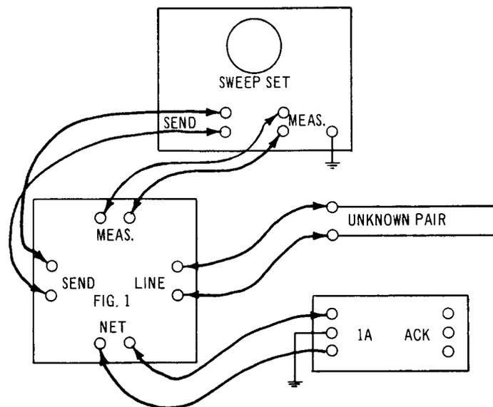
Fig. 3 – Arrangement for Return Loss Technique
