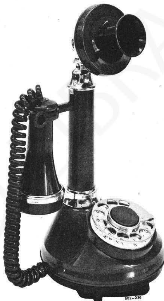
Fig. 1 — 420-Type Candlestick Telephone Set
