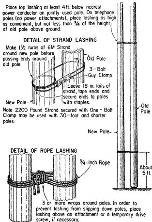
3.03 In order to place the upper lashing, climb the new pole. Do not, under any circumstances, work from the old pole until both upper and lower lashings have been completed. Rope lashings should be used only where the old pole is to be removed within a reasonable period of time (usually a few days) or where there might otherwise be an electrical hazard in passing the sling around the poles.
