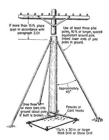
Place clove hitch on bar driven into ground. Draw rope taut and place clove hitch on handle of each peavy or cant hook.
