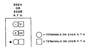
\*If circle or box symbol does not contain a terminal number, the terminal is not a terminating point on that particular key telephone unit.
