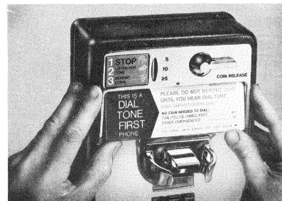
FIG. 2 - Installing Instruction Cards (All 1-Type and Current Production 2-Type)
