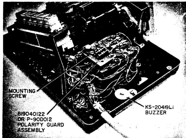
Fig. 3—819040122 (P-90D012) Polarity Guard Assembly Installed in 2662A1M Telephone Set Base
