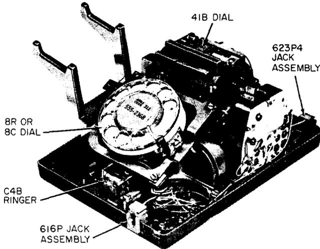
**Fig. 2—660A1M Telephone Set Base**
