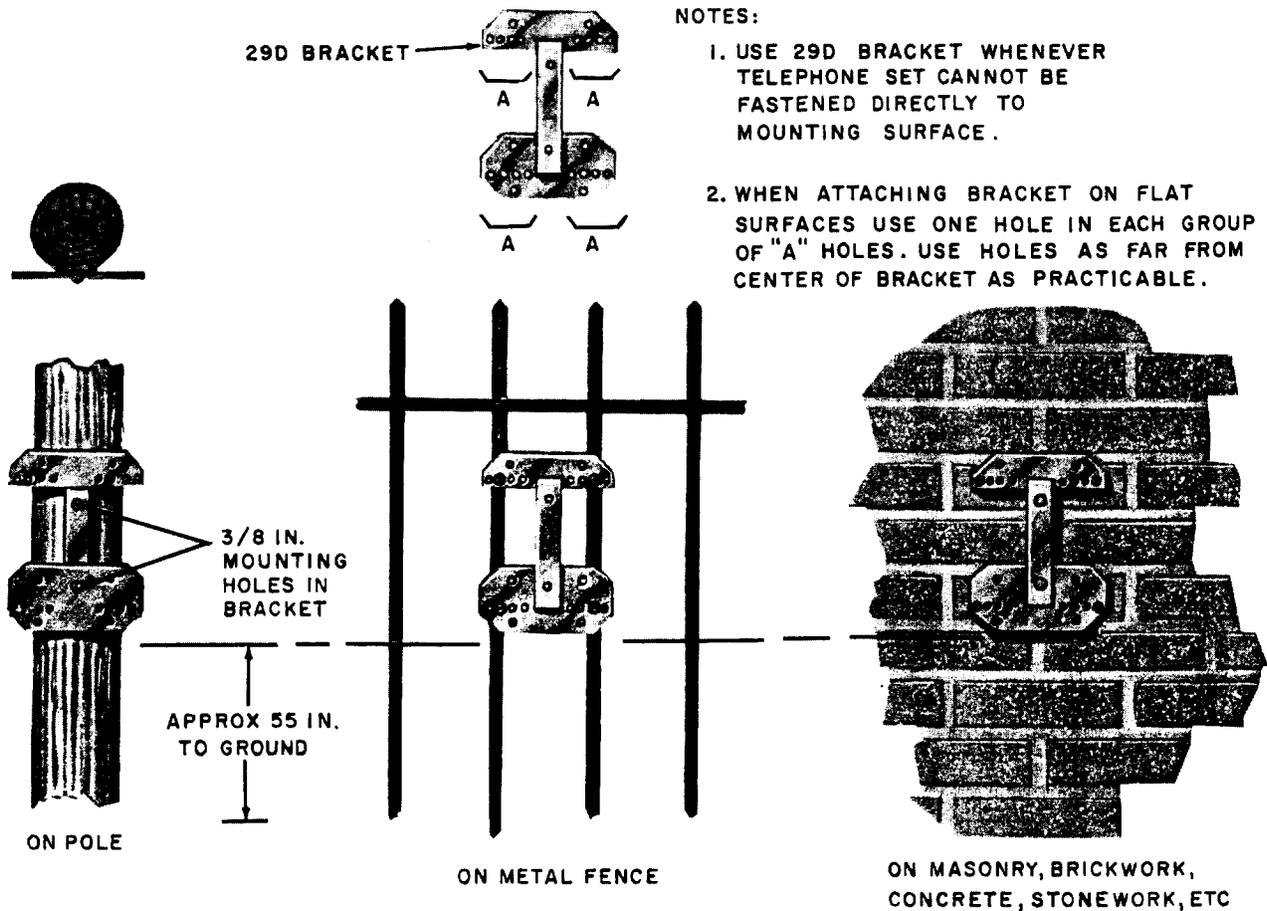
Fig. 2—29D Bracket Mounted on Various Surfaces
