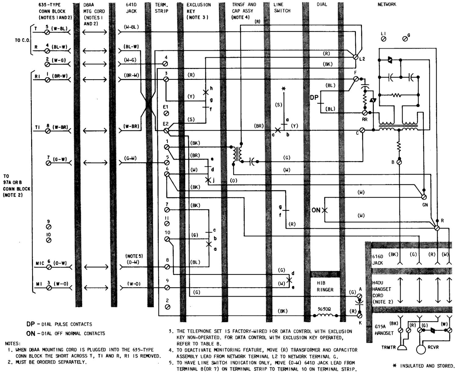
Fig. 4—503CM Telephone Set, Connections
