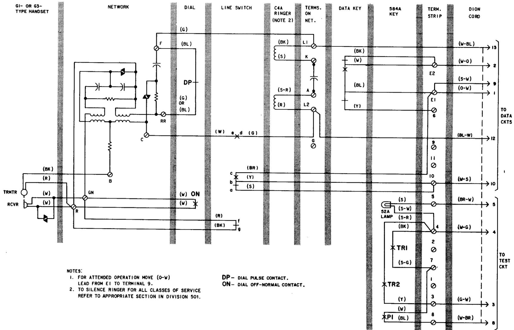
Fig. 5—513B (MD) Telephone Set, Connections
