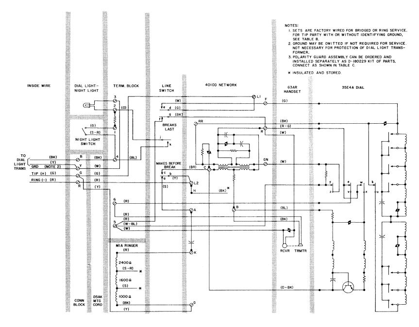
Fig. 1 — 2702B Telephone Set, Connections
