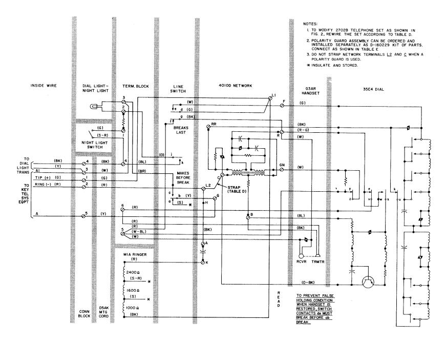
Fig. 2 — 2702B Telephone Set, Wired For Use With 1A1 or 1A2 Key Telephone System
