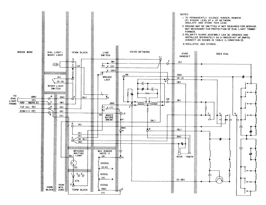
Fig. 3 — 2702D Telephone Set, Connections
