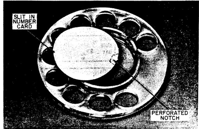
Fig. 4—Method of Placing Number Card in Current Plastic Fingerwheel
