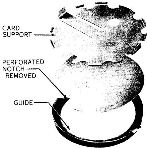
Fig. 2—Method of Placing Card in Holder
