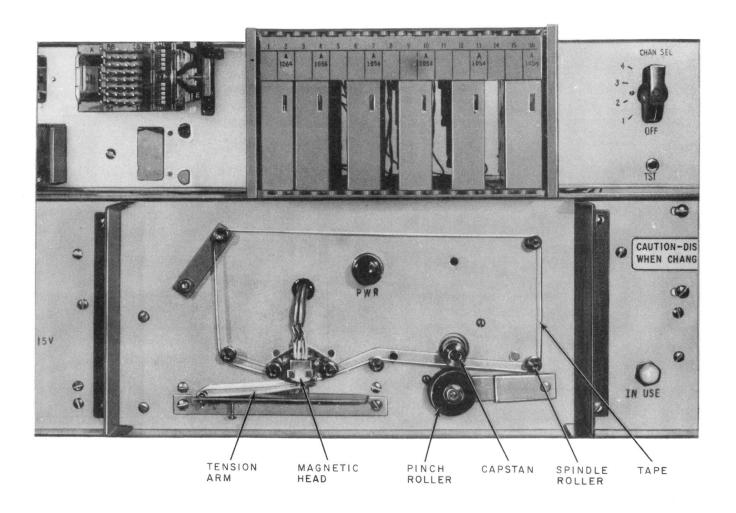
Fig. 2—12A Announcement System (Front Door Removed)
