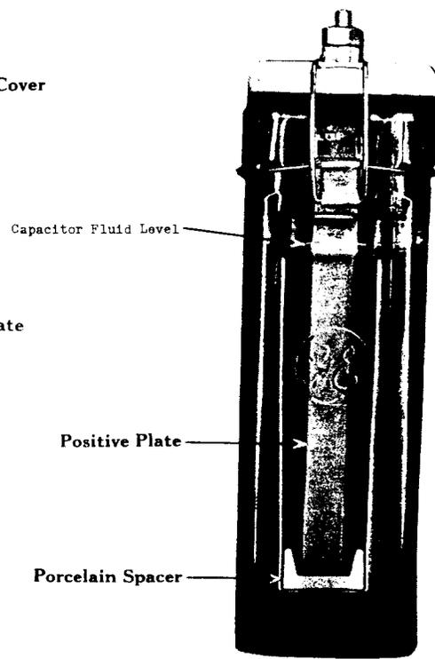
Fig. 4 - 101 Type Electrolytic Capacitor Assembly, End View
