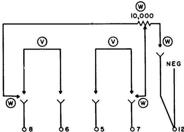
Fig. 5 - Connection Data for Remote Gain Control for KS-16754 Amplifier
