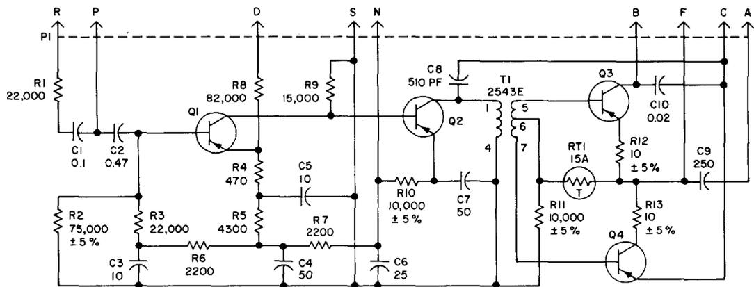
Fig. 3—KS-16728 L1 Amplifier, Schematic
