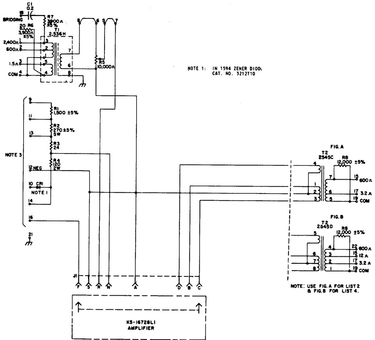
Fig. 7 - KS-16754, List 2 and 4 Amplifiers, Schematic
