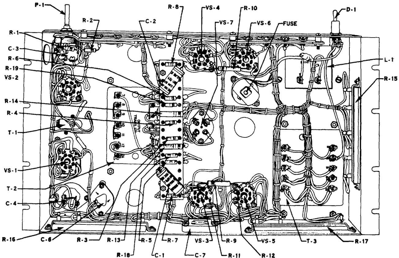
Fig. 1 - Bottom View of 118A Amplifier
