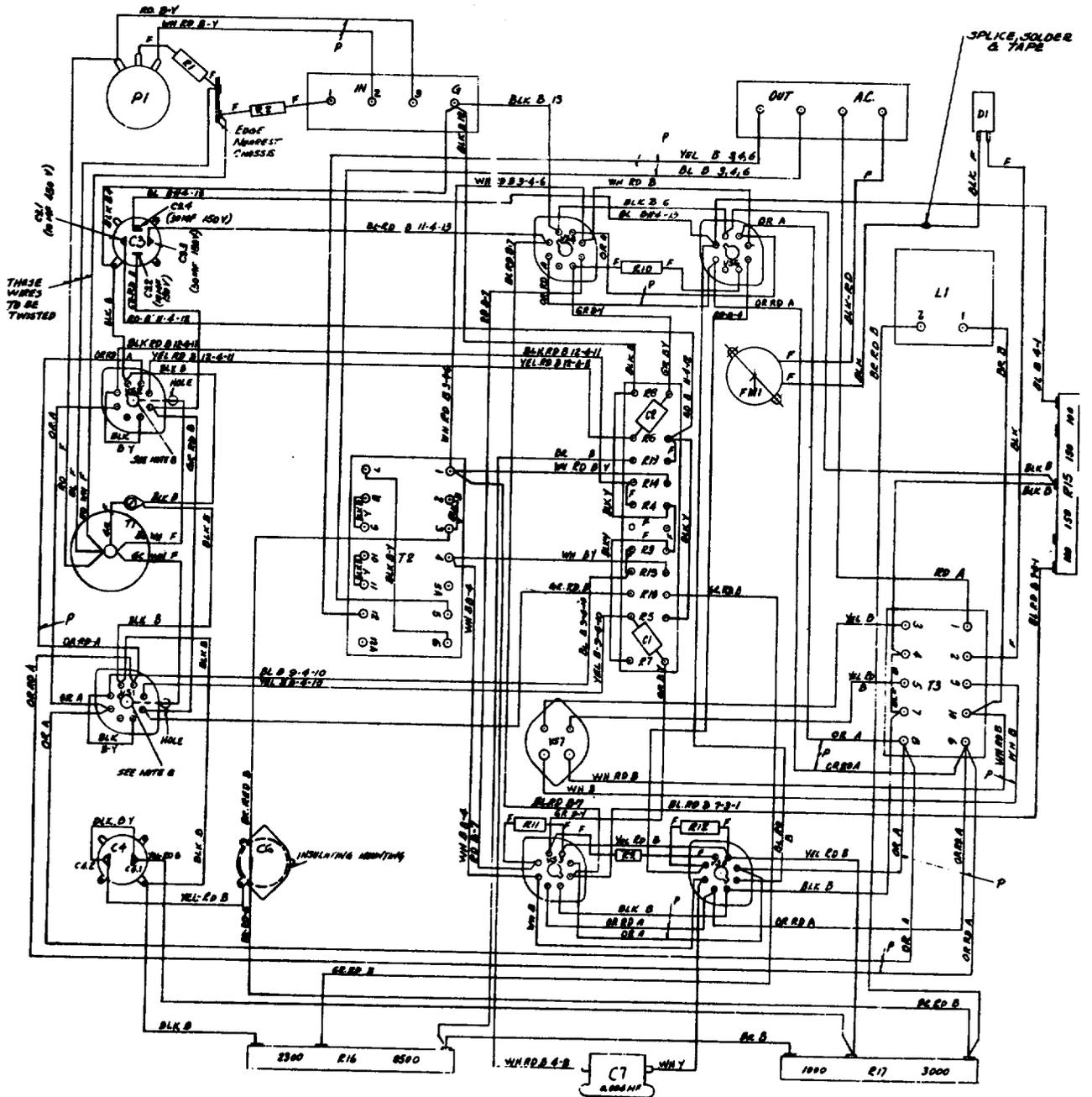
Fig. 3 - Wiring Diagram of 118A Amplifier
