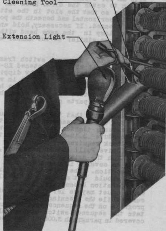
Fig. 8 - Method of Cleaning Adjacent Surfaces of "A" and "B" Cams
