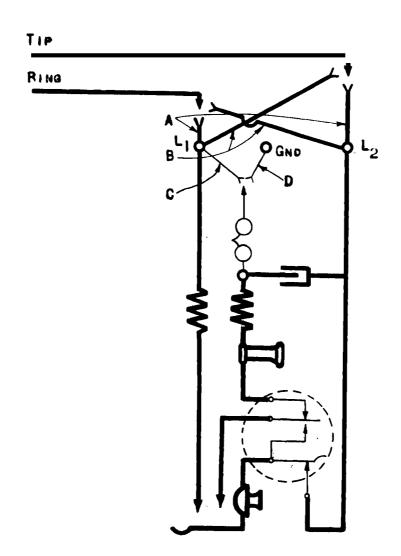
NOTE: ON INDIVIDUAL LINES USE "A" AND "C" WIRING.
