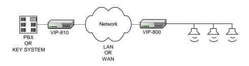
In this example, the VIP-810 was connected to the data network jack already installed and now the network connected telephone can reach into the existing Valcom Page Controller to access all call priority paging. This configuration could be used at a guard shack where network access is available, but not telephone.
