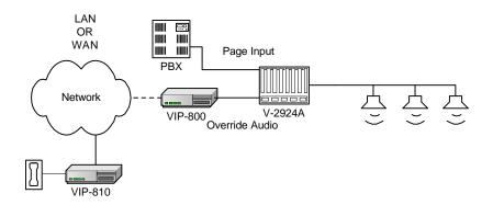
In this example, the VIP-810 and VIP-800 are connected to the data network as stand alone paging. This could be installed where network access is available, but not paging.
