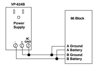
When installing Valcom one-way amplified speakers, connect the -24V and ground terminals of the speaker to the power supply (-) and (+) terminals respectively.
