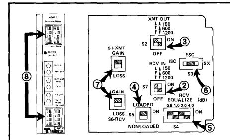
**1** Refer to the CLR and determine the following: receive-channel input impedance, transmit-channel output impedance, receive-channel equalization, the type of facility the module interfaces, and whether gain or loss is required in the receive and transmit thannels. Once these requirements are known, proceed to step 2 and perform the remaining preliminary alignment steps in numeric order.
