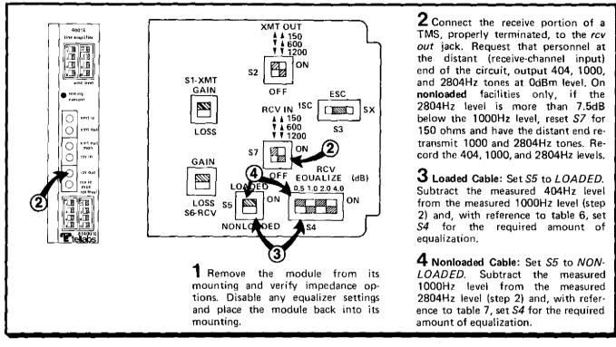
figure 14. 4001E frequency-response measurement and cable-loss data
