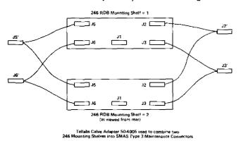
figure 7. Interfacing Two 246 Mounting Shelves into SMAS
