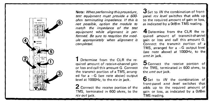
figure 12. 4001E gain adjustment procedure
