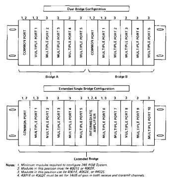
figure 5. Physical arrangement of 246 System modules (front view)
